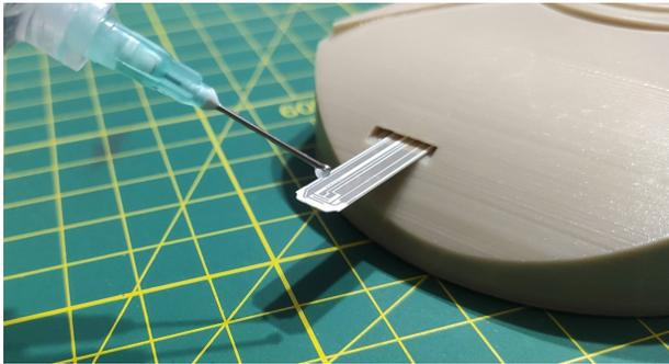
**Figure 4:** Image of the moment in which the biological sample of viral rhinopharyngitis extracted is placed on the electrode.
