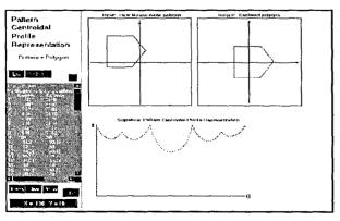
Given a pattern (polygon) in input image, this software detects its Centroid (geometric center), then displaces the whole pattern in such a way as to place its centroid in the origin of coordinates (0,0),
